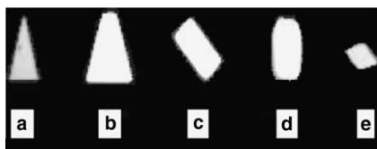
Figure 6. Grey scale images of crystal shapes obtained in the different experiments. Projected images of (a) faces (110), (100) and (1 \bar{1} 0) at supersaturations of 1.95 and 2.34, (b) faces (110), (100) and (1 \bar{1} 0) at a supersaturation of 3.15, (c) face (011) of a plate-shaped crystal, (d) face (011) of a tomahawk crystal and (e) face (010).
